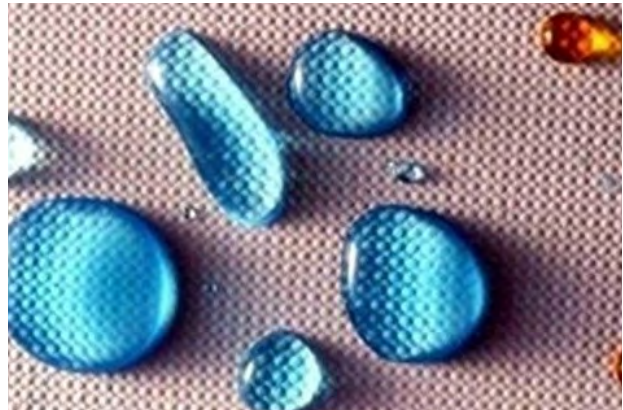
Figure 5 Water droplets on hydrophobic fabric
